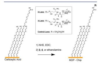
**Figure 2.** Synthesis of the MDP chip. A mixed SAM consisting of 1 mol % hexa(ethylene glycol)carboxylic acid  $[(EG)_6CO_2H]$ -terminated thiol in tri(ethylene glycol)  $[(EG)_3OH]$ )-terminated thiol was prepared. The carboxylic acid groups were then activated with NHS and EDC to form NHS esters. Displacement of NHS esters with the amino groups of MDPs formed amide bonds. Excess NHS esters were deactivated with ethanolamine.
